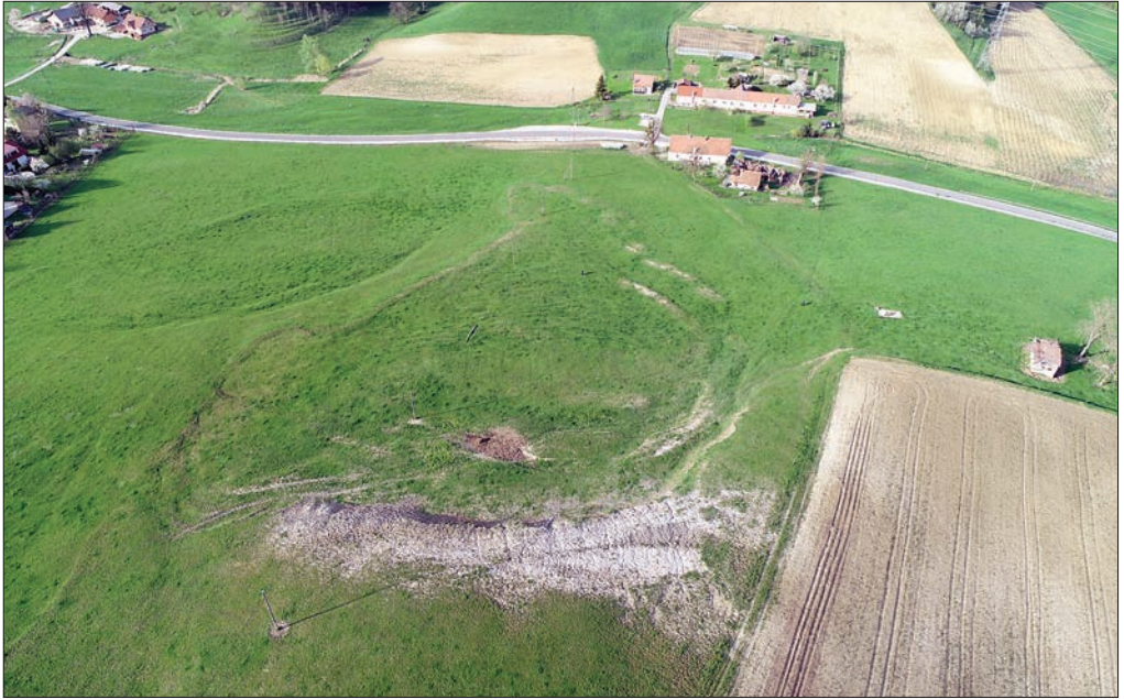
Figure 6: After trees were cut down and the roadside drainage was altered near Šentilj in Slovenske Gorice Hills, the area became prone to landsliding.
