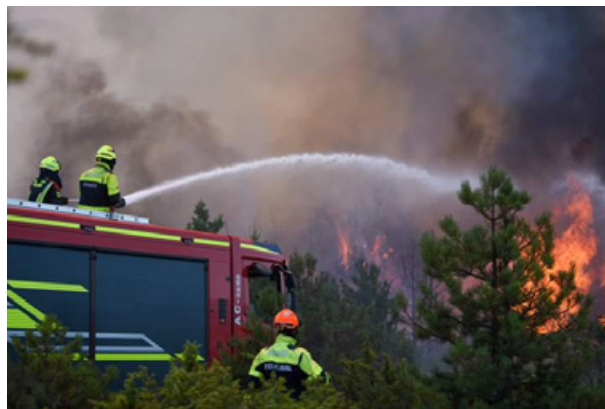
Slika 7: Gašenje vršnega požara z vodnim monitorjem na gozdni cesti Figure 7: Fighting a crown fire with a water monitor on a forest road
