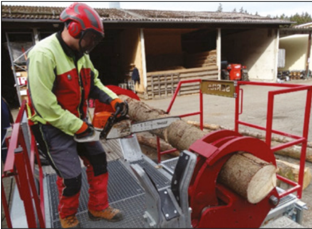
Slika 15: Simulator za ustvarjanje napetih vlaken v hlodovini (vir: Gasilska šola) Figure 15: Simulator for reproducing the effect of strained fibres in timber (Source: Firefighting School)
