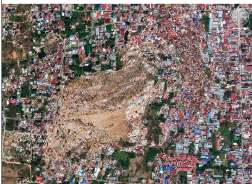
Figure 6: A satellite image shows the Balaroa neighbourhood of Palu, Indonesia, provided (a) on 17 August 2018 and (b) on 1 October 2018; before and after the earthquake and subsequent tsunami caused heavy damage to the area. A comparison of the pictures shows that many houses disappeared under a sea of brown mud, after the strong earthquake tremors liquefied soil underneath them and buildings' foundations lost support. (Source: https://abcnews.go.com/International/death-toll-1200-indonesian-quake-tsunami-catastrophe/story?id=58225541 )
