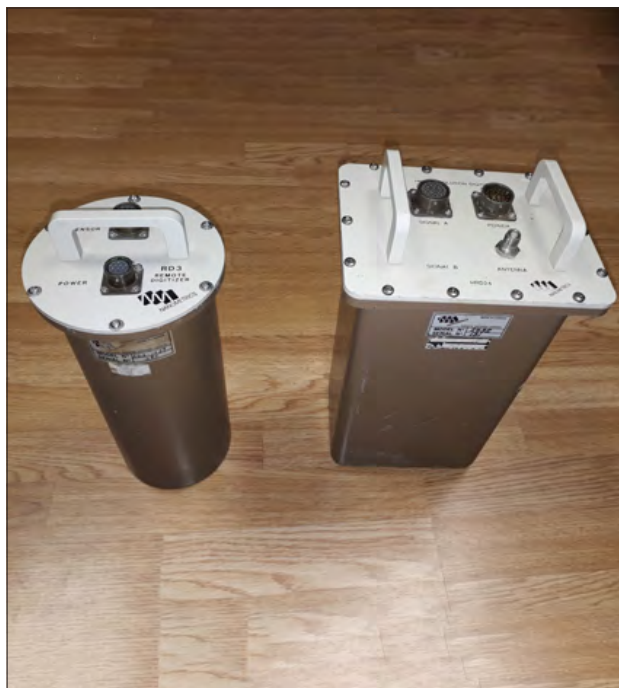
Slika 6: Zajemalna enota RD-3 (levo) in zajemalna enota HRD-24 (desno) [avtor: I. Tasič] Figure 6: Acquisition unit RD-3 (left) and acquisition unit HRD-24 (right) [Author: I. Tasič].
