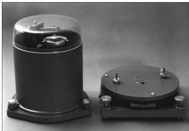
Slika 2: Seizmoskop WM-1 (levo) in podnožje, na katerem se je opravljala kalibracija (desno) Figure 2: WM-1 seismoscope (left) and the base, on which the calibration was performed (right).
