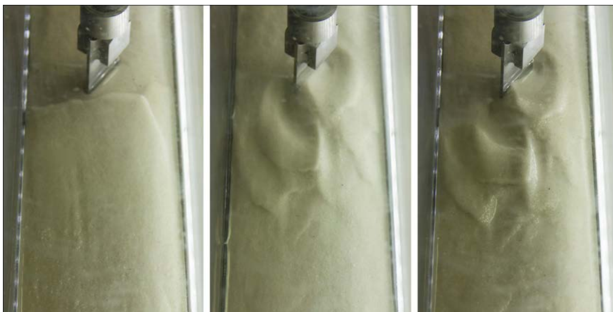
Slika 3: Primer vpliva mostnega opornika (ovire) na transport sedimentov Figure 3: Example of the influence of a pier on sediment transport.
