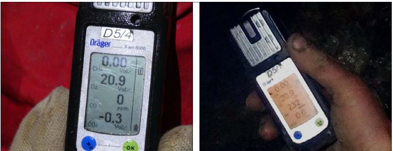
Slika 8: Detektor plinov; a) pred vrtnjem in b) primer prikaza plina CO po nekajminutnem vrtnju z bencinskim vrtnikom v slabo zračeni jami [232 ppm] (foto: M. Merela) Figure 8: Gas detector; a) before drilling and b) a case of the CO gas concentration after a few minutes of drilling with a petrol hammer drill in a poorly ventilated cave [232 ppm]. (Photo: M. Merela)
