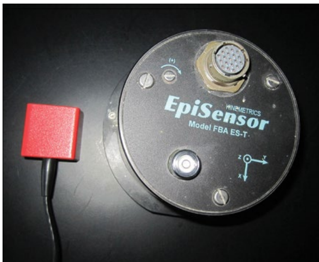
Slika 1: Pospeškometer JW 24F14 (levo, oranžni) in profesionalni pospeškometer EpiSensor (desno) Figure 1: Accelerometer JW 24F14 (left, orange) and professional accelerometer EpiSensor (right).
