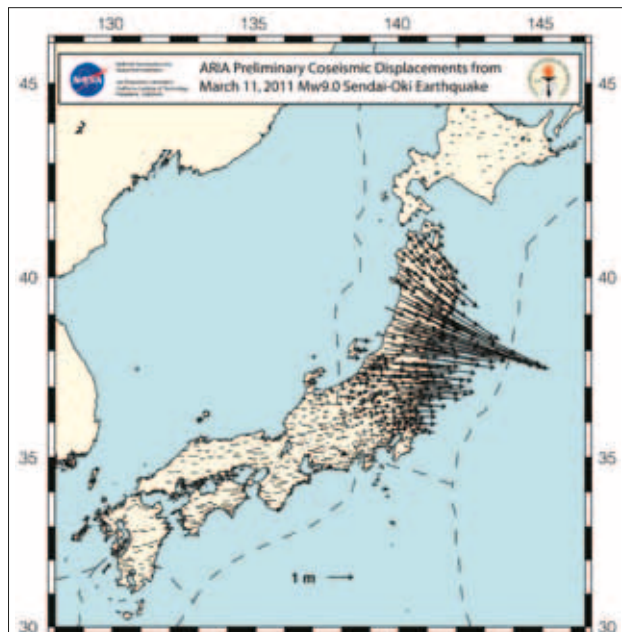
Slika 5: Obpotresni premiki ozemlja proti vzhodu, izmerjeni z GPS-opazovalnicami Figure 5: Co-seismic displacements of land towards the east, recorded with GPS stations.
