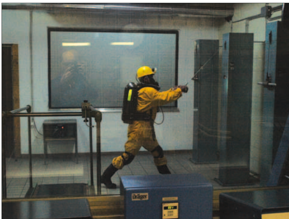
Slika 5: Psihofizično testiranje reševalcev v dimni komori s telemetrijo ob navzočnosti zdravnika (foto: D. Reberčnik) Figure 5: Psychophysical testing of rescue workers in a smoke chamber in the presence of a physician and with the use of telemetry (photo: D. Reberčnik).
