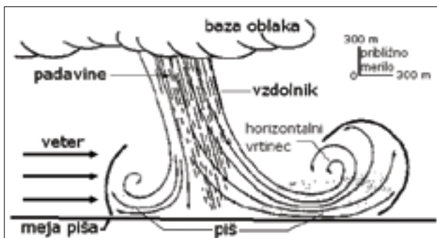
Slika 1. Skica močnega vzdolnika in asimetričnega nevihtnega piša. Prirejeno po http://www.srh.noaa.gov/jax/events/windshear.html Figure 1. Pattern of downburst and asymmetric thunderstorm outflow. Adapted from http://www.srh.noaa.gov/jax/events/windshear.html
