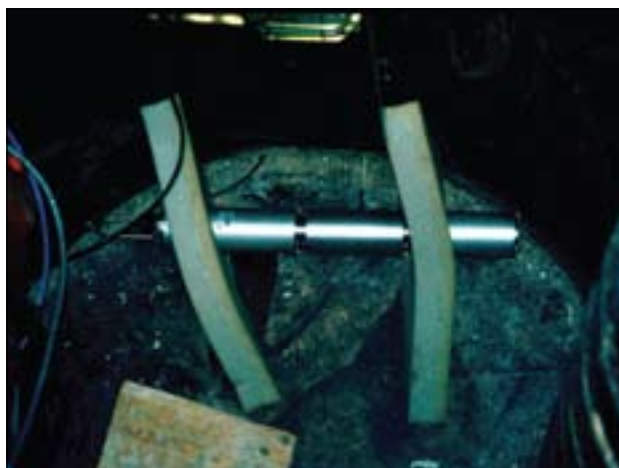
Slika 2. Seizmometer CMG 40TBH v jaški potresne opazovalnice pred namestitvijo v vrtino. Figure 2. CMG-40TBH seismometer in a vault at the seismic station before installation in the borehole.
