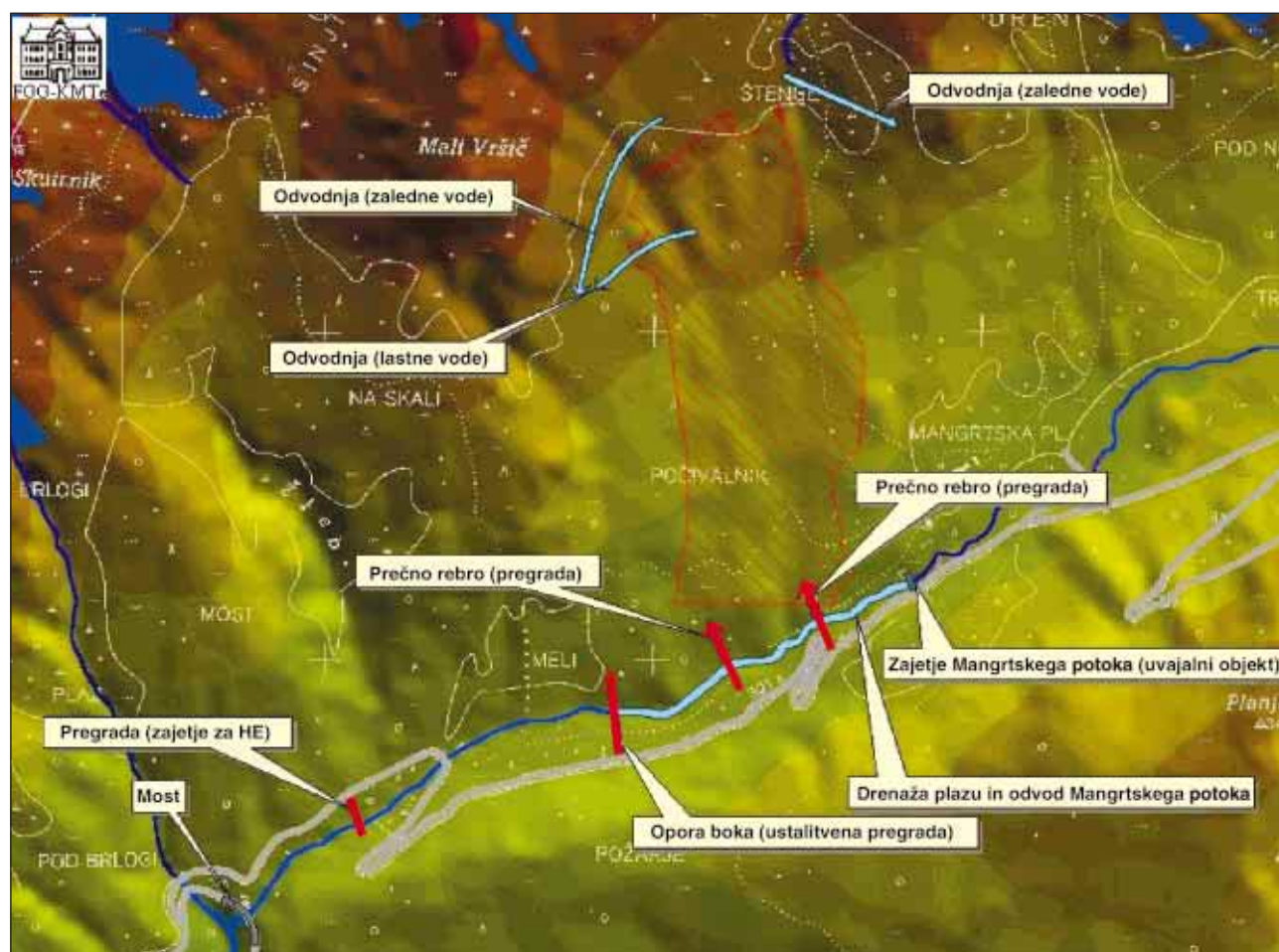
Slika 6. Zasnova interventnih posegov in njihove nadgradnje v možne sanacijske ukrepe (FGG-KMTe) Figure 6. Concept of intervention measures and their upgrading into possible consolidation measures (FGG-KMTe)
