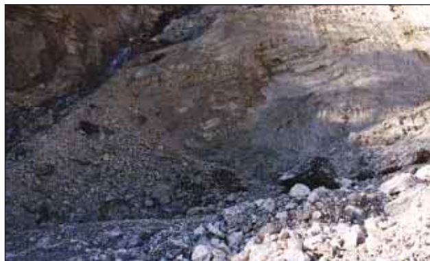
Slika 4. Vpadi laporja na severozahodnem odlomnem robu plazu (foto: B. Petkovšek) Figure 4. Marl intercalations in the northwestern fracture zone of the landslide (photo: B. Petkovšek)
