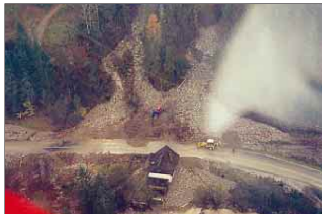
Slika 10. Hudournika Grabnarjev potok in Suhi potok sta ogrozila stanovanjsko hišo in z naplavinami povsem zasula regionalno cesto Luče (Sestre Logar). (foto: T. Jeršič) Figure 10. The torrents of Grabnarjev potok and Suhi potok endangered a residential building and completely buried the Luče – Sestre Logar regional road (photo: T. Jeršič)
