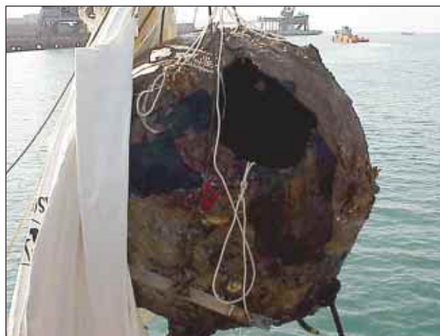
Slika 2. Morska mina EMC 300, t. i. ježevka, med dvigom iz morja. Na levi strani ob mini visijo podvodna padala, ki so služila za dvig in prevoz po morju (foto: UO Koper) Figure 2. EMC-300 sea mine is being lifted from the sea. To the left, alongside the mine, are underwater parachutes used for lifting and sea transport (photo: UO Koper)
