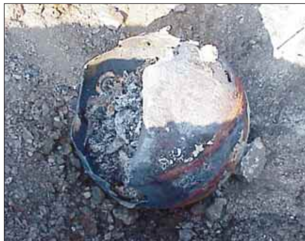
Slika 5. Tako izgleda mina po uničenju z izžiganjem vsebine (foto: UO Koper) Figure 5. A mine after being neutralized by evaporation (photo: UO Koper)
