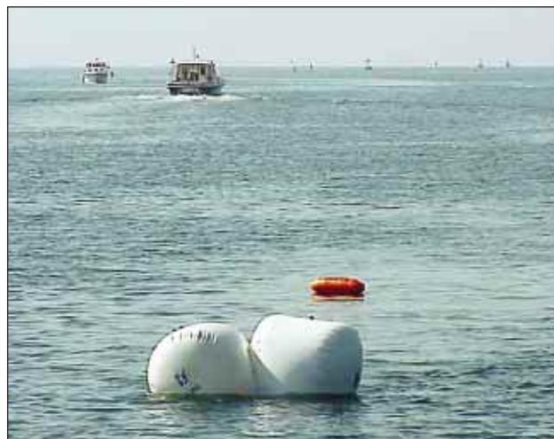
Slika 6. Prvič preizkušen način prevoza morskih min s podvodnimi padali. Mina je med prevozom 2 do 3 m pod morsko površino (foto: UO Koper) Figure 6. Transport of sea mines with underground parachutes, first tested in practice. The mine is transported 2-3 metres below the water surface (photo: UO Koper)
