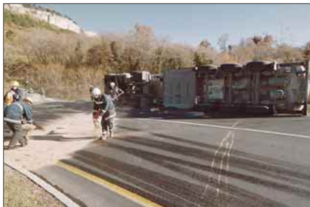
Slika 2. Začetno čiščenje madeža s posipavanjem absorpentov (foto: FPA Koper) Figure 2. Initial removal of spill by the dispersion of absorbents (photo: FPA Koper)
