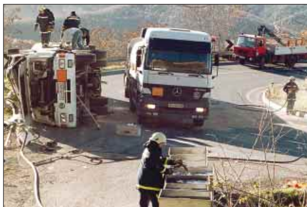
Slika 3. Gasilci prečrpavajo gorivo v za to namenjene 600-litrne posode (foto: FPA Koper) Figure 3. Firefighters repumping fuel into specially designed 600 l vessels (photo: FPA Koper)
