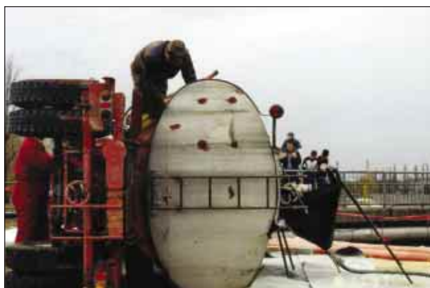
Slika 11. Pripadniki PIGE Nafta Lendava poskušajo zatesniti poškodovano priklopno avtocisterno in preprečiti nadaljnje iztekanje nevarne snovi; Lendava, 9. 11. 1997 (foto: S. Jauk) Figure 11. Members of the Nafta Lendava Industrial Firefighting Unit attempting to seal a damaged road tanker and prevent the further spillage of hazardous substance; Lendava, 9 November 1997 (photo: S. Jauk)
