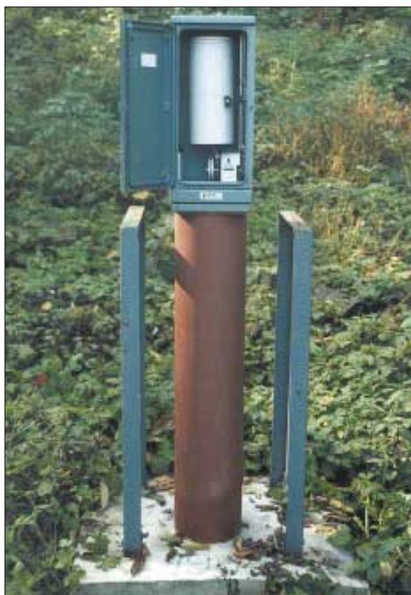
Slika 3. Merilno mesto višine gladine podzemne vode S-3567 Breg (arhiv HMZ) Figure 3. Groundwater level observation station S-3567 Breg (courtesy of HMZ)
