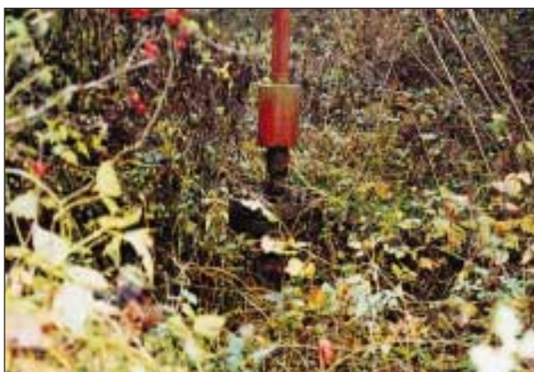
Slika 3. Opuščena nesanirana vrtina Pg-83 na naftno-plinskem polju Petišovci – globoko (foto: M. Smodiš) Figure 3. Abandoned, unrehabilitated Pg-83 well, Petišovci – globoko oil/gas field (photo: M. Smodiš)
