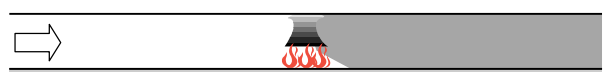
Slika 1. Razvoj dima pri požaru v predoru Figure 1. Smoke development in a tunnel fire
