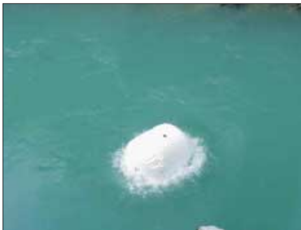
Slika 8. Dvigovanje plinske granate na površje s pomočjo zračnega balona (foto: M. Lampret) Figure 8. Lifting a gas shell to the surface with the help of an air balloon (photo: M. Lampret)
