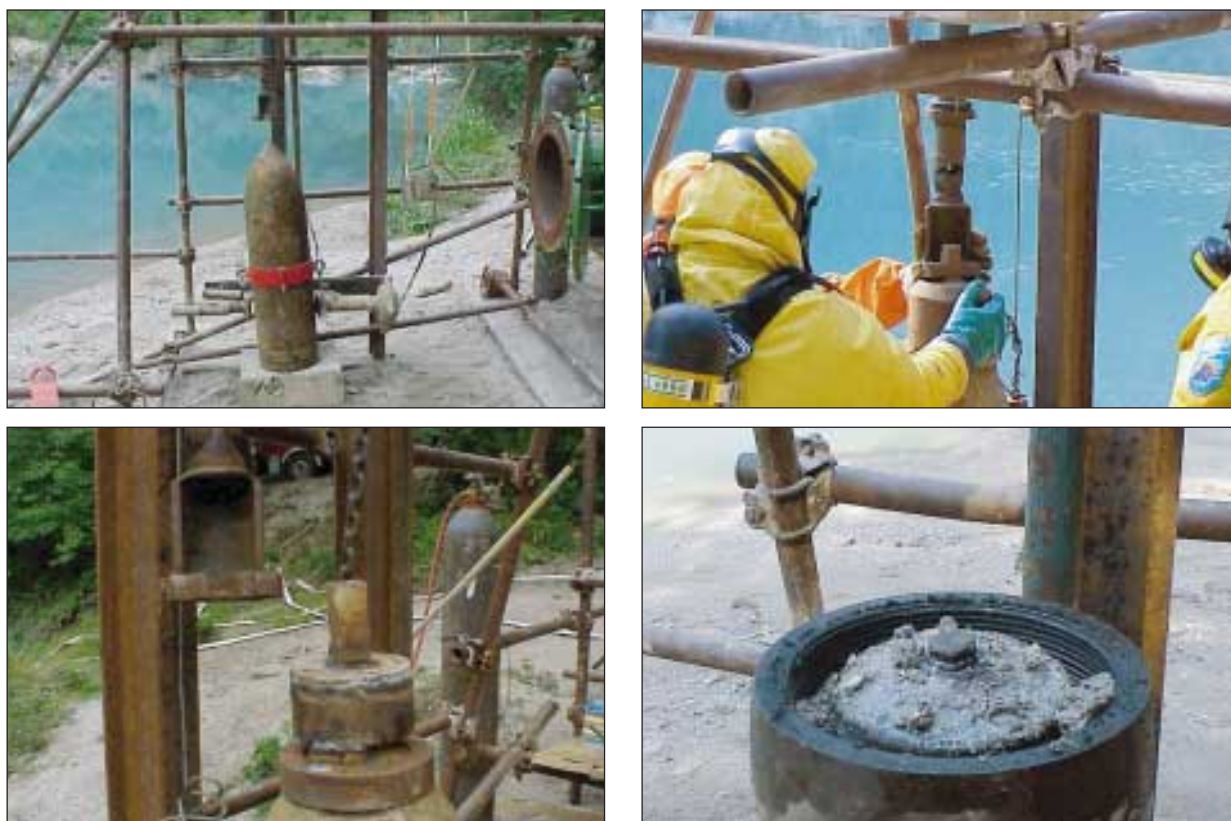
Slika 10. Postopek odpiranja granat (foto: M. Lampret) Figure 10. The process of opening shells (photo: M. Lampret)
